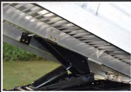
Cross Member-less floor for Lower Center of Gravity
